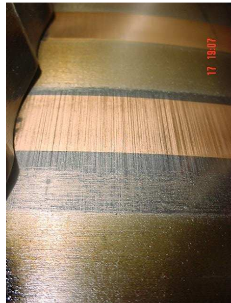
Initial wearing in of copper band on the piston skirt of Unit 4. Pic 4 – Ship A (Inspection on 17 th March 03)
