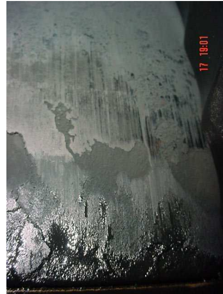
Deposits on Unit 4 piston top land abrading the liner wall. Pic 3 – Ship A (Inspection on 17 th March 03)
